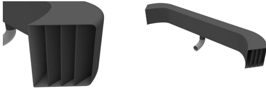
Fig-3.5.i Air Intake System
