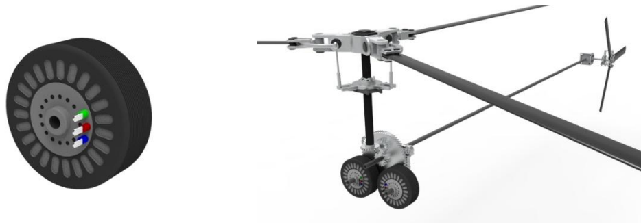
Fig-2.4.i: EMRAX 268 Motor Integration With Main and Tail Rotor.
